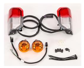
Includes turn signals (front and rear), reverse lights, and hazards
